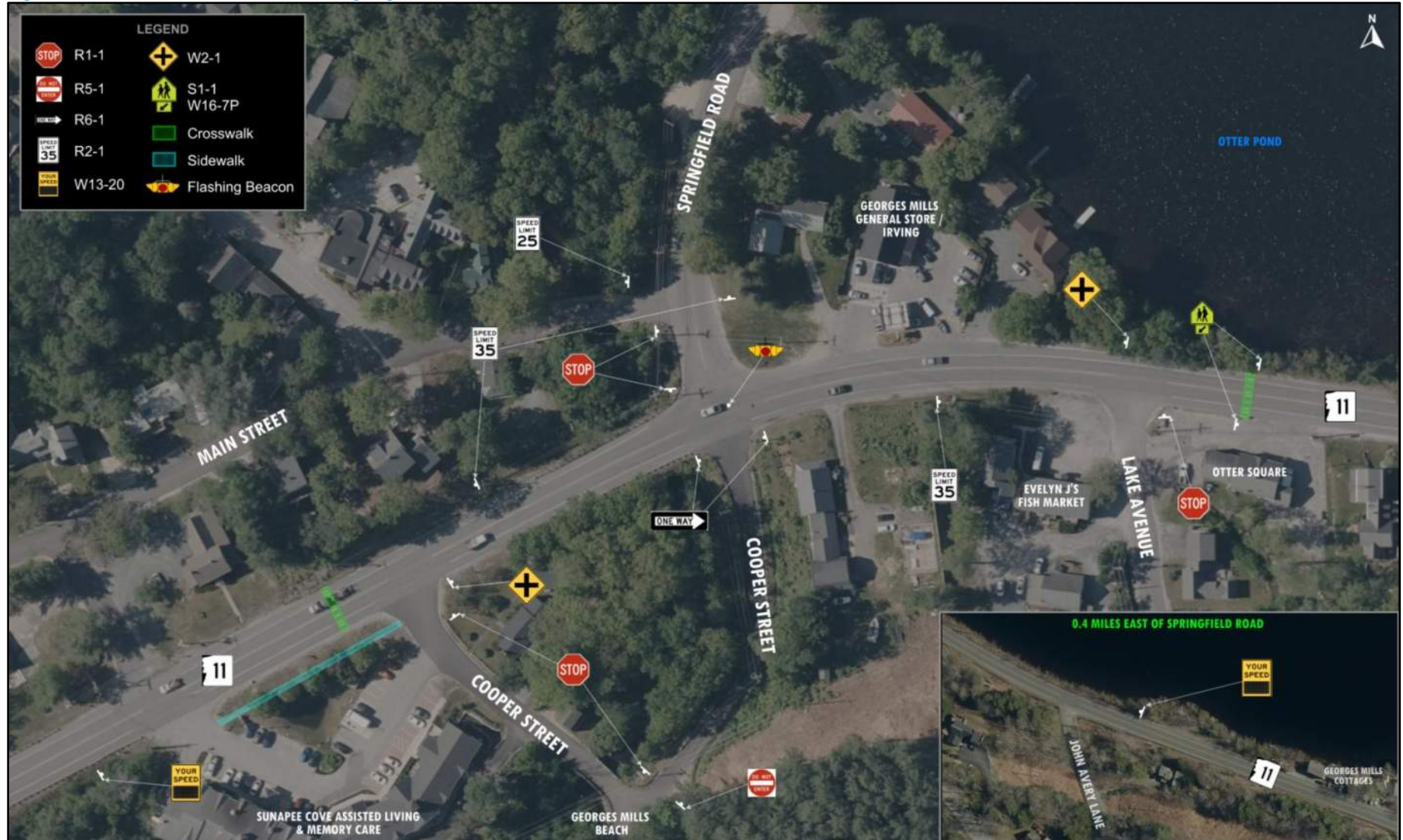
Figure 4 - RSA Intersection Control & Signage
